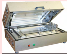
Fig. 1 : Irradiation device for UVC treatment of PCs
