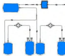
**SPV system** : filtration of the aphaeresis unit with Plasmaflex MB Pill dissolution and distribution in 2 units > illumination > MB removal with Blueflex
