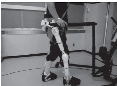
**Figure 4:** Gait training using the robot suit HAL<sup>®</sup> with a walking device and a harness for safety.
