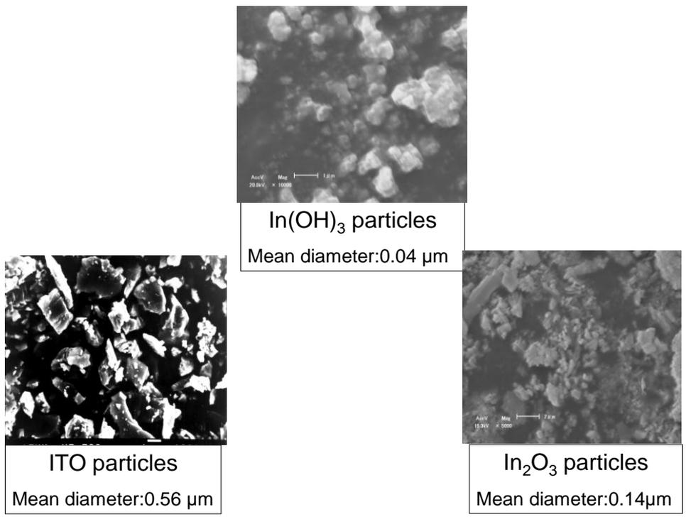
Fig.1 Scanning electron micrographs of In(OH)<sub>3</sub>, ITO and In<sub>2</sub>O<sub>3</sub> particles
