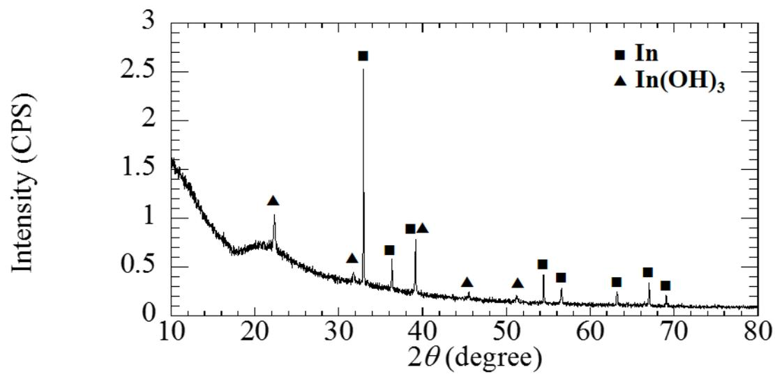
Fig. 5. XRD pattern of synthesized nanoparticles.
