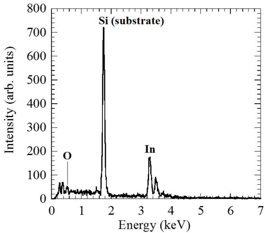
Fig. 4. EDX spectrum of synthesized nanoparticles.
