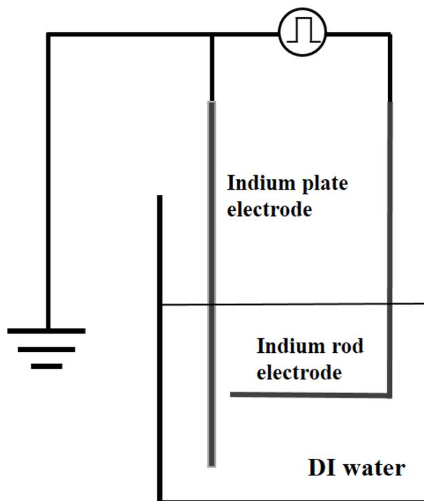
Fig. 1. Schematic of experimental setup for synthesis of indium-containing nanoparticles using pulsed electrical discharge plasmas in DI water.
