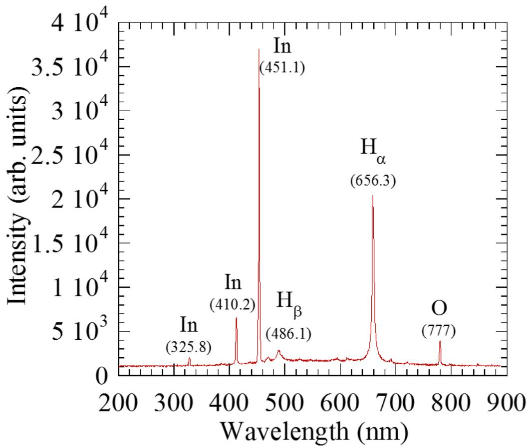
Fig. 2. Optical emission spectrum of pulsed electrical discharge plasma in DI water.
