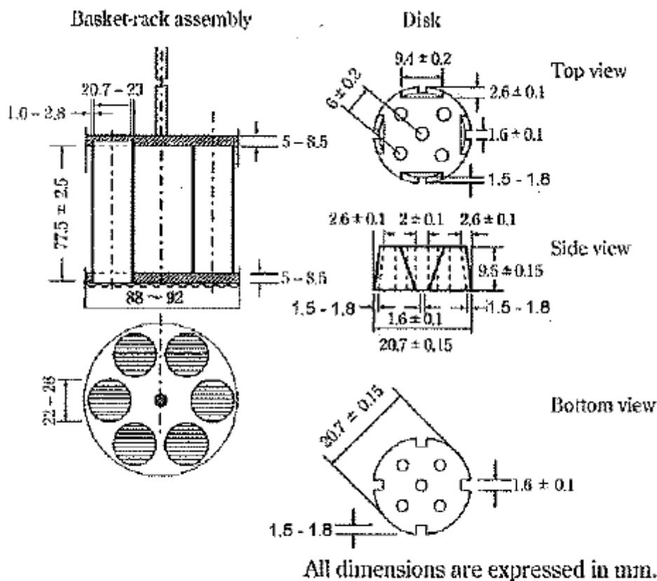
Fig. 6.09-1 Disintegration apparatus
