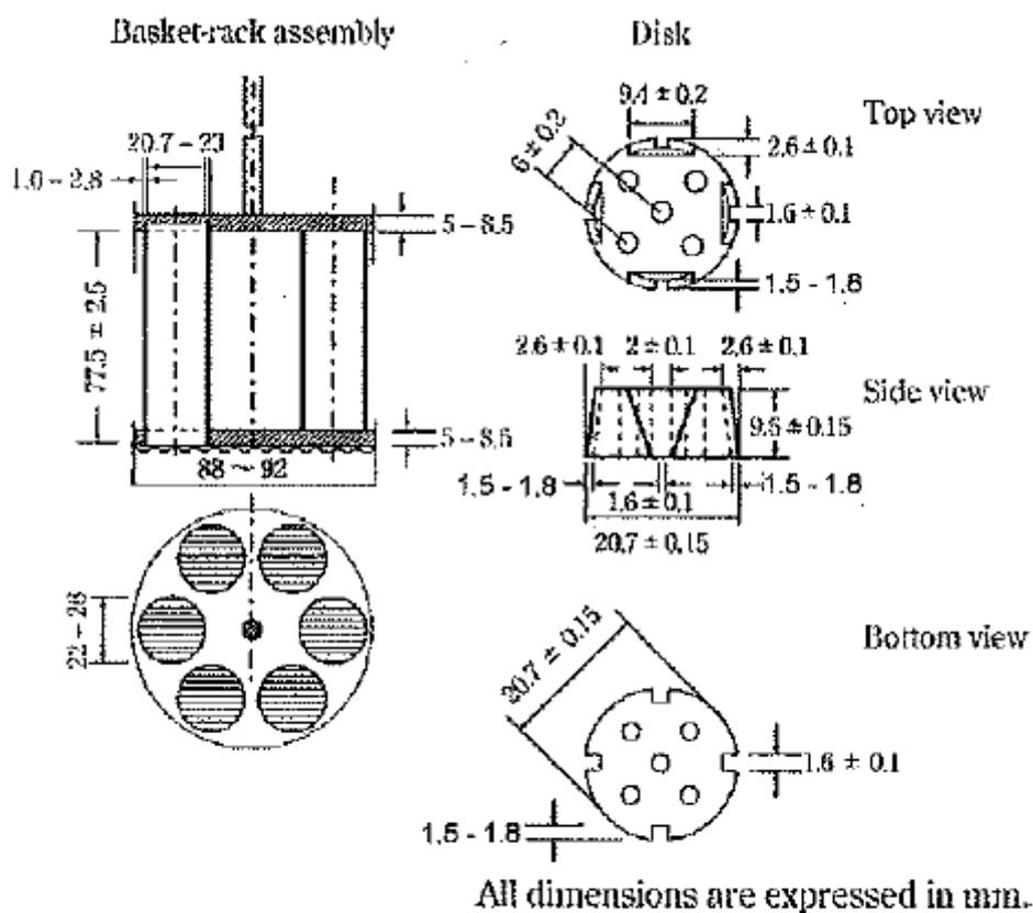
Fig. 6.09-1 Disintegration apparatus
