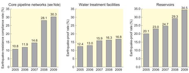
(Note) The figures indicate the percentage of pipes that were earthquake-resistant (earthquake-proof rate) up to FY2006 and the percentage of pipes that meet earthquake-resistance standards (earthquake-resistant pipes + non-earthquake-resistant pipes but which are situated in better ground and are therefore considered to be earthquake-resistant) (earthquake-resistance compliance rate)
