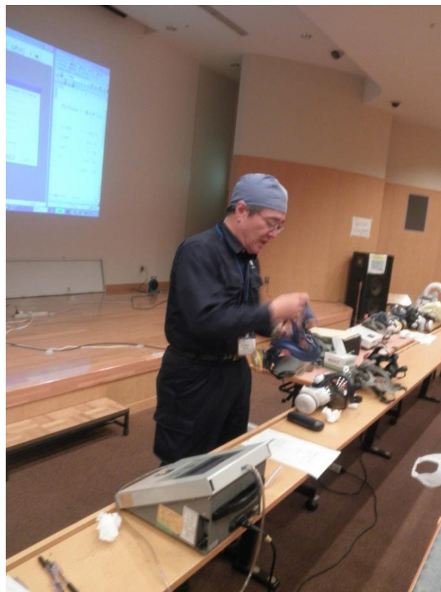
Photo 2 Demonstration by an expert from the Institute. He first explained the intention of the investigation, actually conducted a fitting test and showed the real time leak rate change that occurred according to movement of the body, etc. on the screen in back of him. The device circled in red is the Mask Fitter Tester – MT-03.
