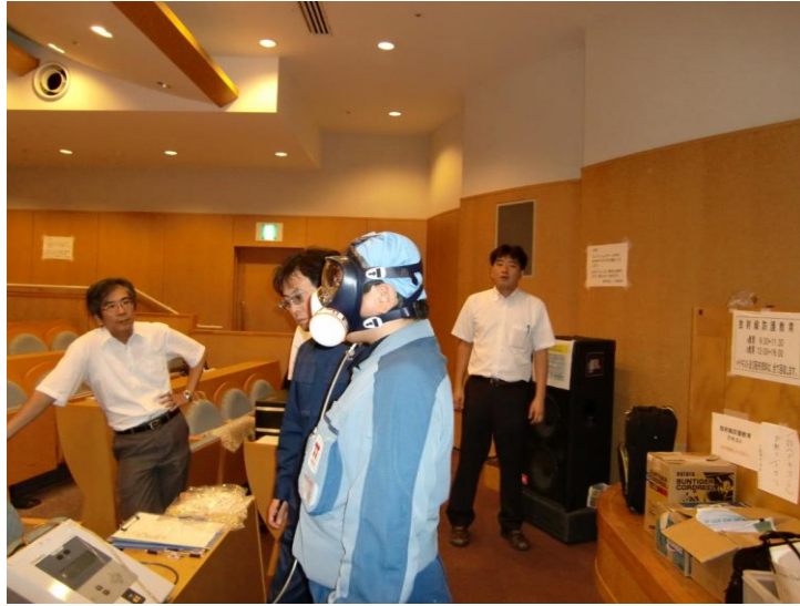
Photo 4 Re-testing the fitting after a subject attached sealing pieces to his eyeglasses.
