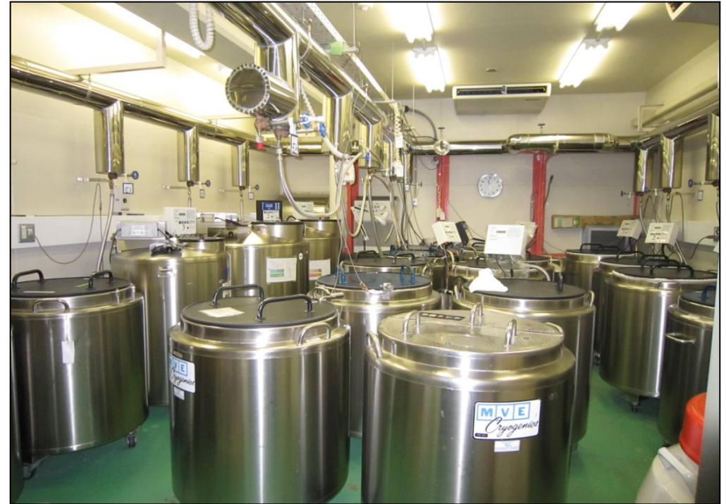
Liquid nitrogen tanks
