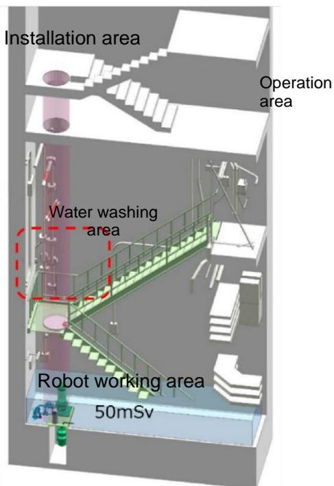
When taking the robot from the basement floor, it was cleaned with high-pressure water.
