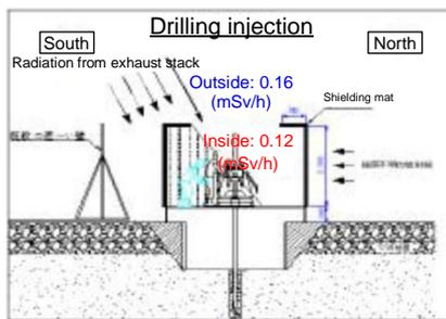
**Fig. 1 Shielding with steel covering**
