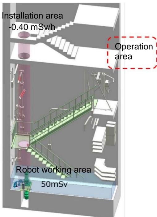
The robot was operated from the operation area in a low dose rate area.
