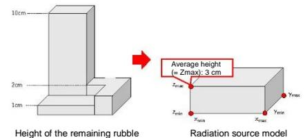
Modeling of the radiation source by averaging the height of the remaining rubble
