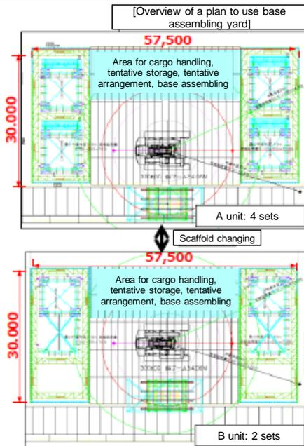
Base steel frames are assembled in a low dose-rate area and carried to a reactor building where the frames are installed. This large unitization construction method can reduce unnecessary exposure.
