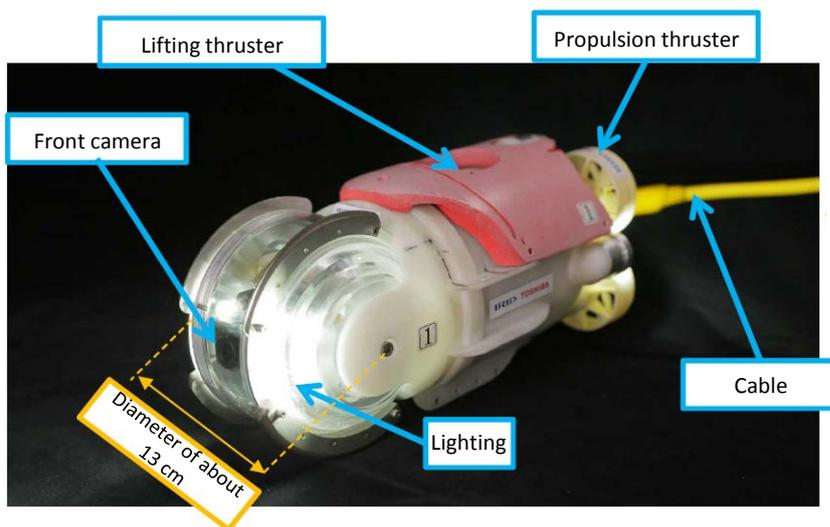
"Unit 3 Reactor: How to Reduce Exposure Dose during Internal Investigation of Reactor Containment Vessel, and Removal and Installation of Fixed Thermometer" (Material provided by Toshiba Energy Systems & Solutions Corporation)
