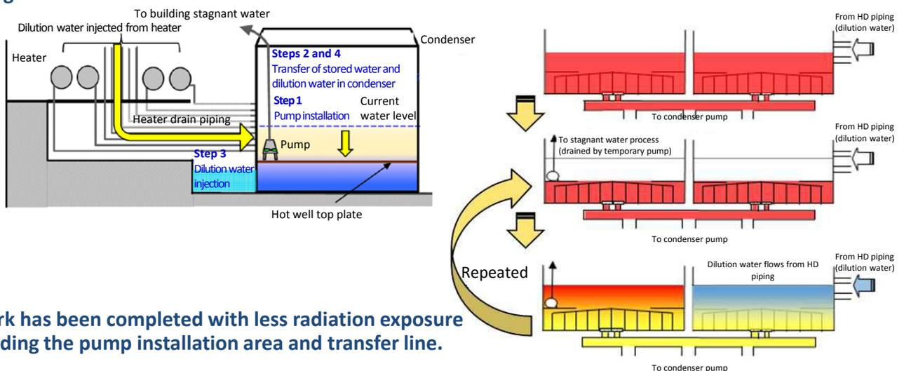
The work has been completed with less radiation exposure by shielding the pump installation area and transfer line.
