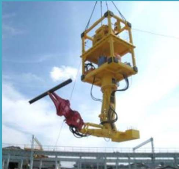
Small steel frame cutter/grippers "Hitokuchi"
