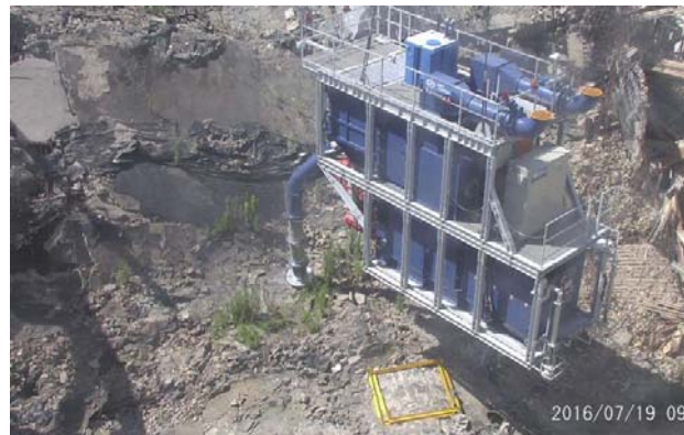
▲ Suction of rubble pieces such as roof blocks using large rubble suction machine
