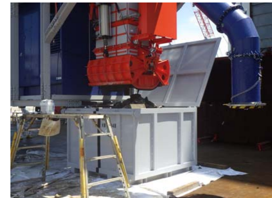
▲ Discharge of small rubble pieces using the large rubble suction machine
