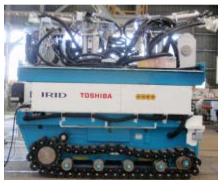
Dry ice-blast decontamination system for the high places *2
