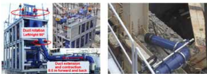
▲ Rubble suction system Decontamination equipment: The equipment was developed to suction up the small rubble pieces through remote operation
