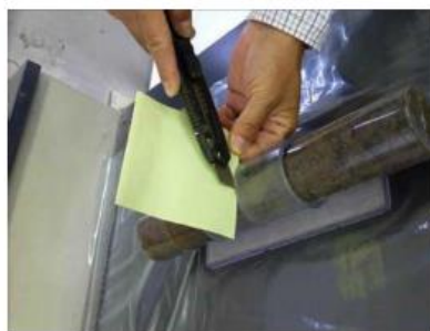
A thin plastic board is inserted between the cut surfaces when a soil sample can collapse easily
