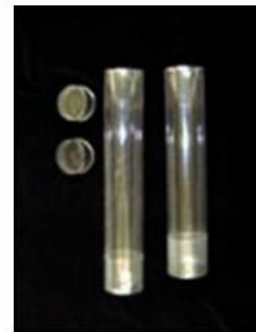
Clear vinyl chloride cylindrical shaped liner
