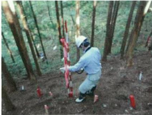
Photo 5. Measuring ambient dose rates after decontamination
