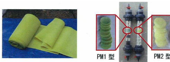
Figure 5: Mass production graft polymer adsorbent (left) and a radiocesium removal filtering device (right).
