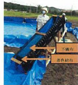
Figure 4: A demonstration test using a decontamination filter
