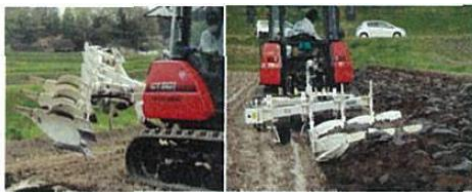
Figure 1: A plow with a jointer attachment (30cm down into the soil, pulled by a tractor): Motomiya City, 9 May.
