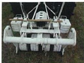
A turf slicer made by Sugano for agricultural purposes was used
