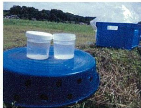
Photo 4: Supernatant water after the solid-liquid separation (radiocesium concentration was less than the detectable level)
