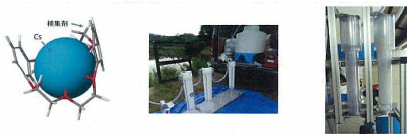
Figure 6: Cesium absorption structure by crown ether adsorbent (left) and a cesium removal device (middle photo, pre-filter; right photo, cyclone separator).
