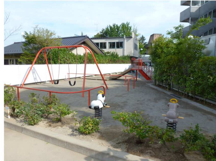
After decontamination Ambient dose rate: 0.8 \mu\text{Sv/h} Dose rate on soil surface: 0.4 \mu\text{Sv/h} (Concrete: 0.2 \mu\text{Sv/h} ) (GM 218 cpm avg., BG 200 cpm)
