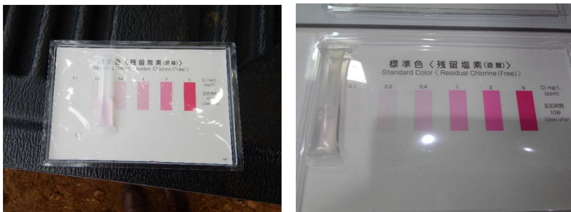
Photo 2.3 Results of Pack Test for Residual Chlorine Left: At Toula Village (PM 2:00), Right: City Center of Neiafu (PM 10:00)
