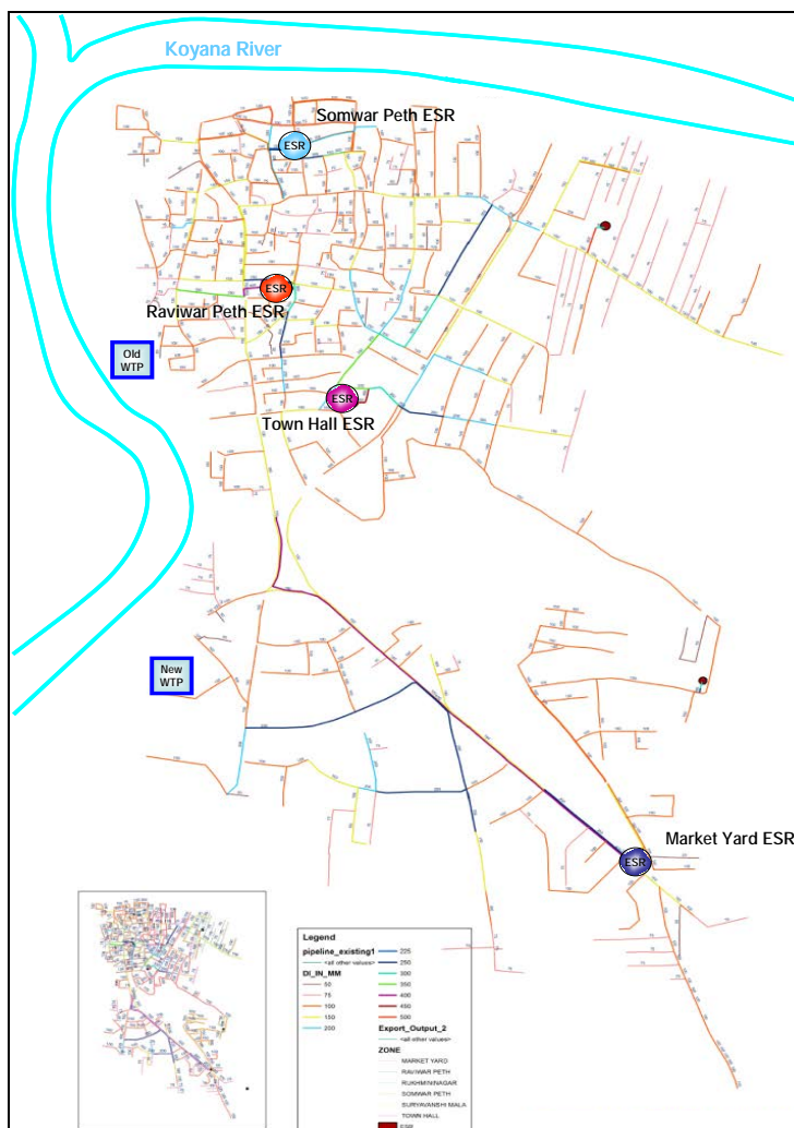
Figure 2-2 Water Supply Facility Location Map
