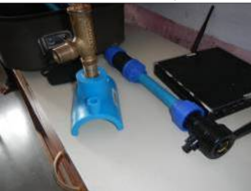
Connection pipe and remote radiowave detective device for water meter used in Malkapur
