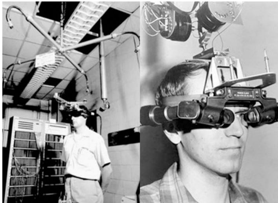
※Ivan Sutherland's first VR Head Mounted Display, The Sword of Damocles (ダモクレスの剣)
