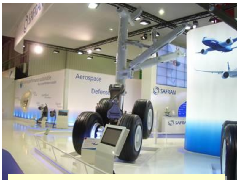
787 Main Landing Gear Assembly
