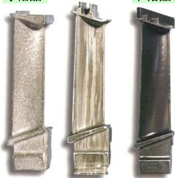
Three common turbine blade casting options balancing cost, yield, and performance: Equiax, directionally solidified, and single crystal alloys
