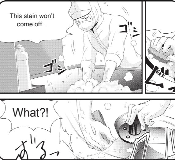
When washing blades by hands, watch out for which way the blade is facing. Also washing with bare hands is very dangerous. Make sure to wear protective gear such as gloves.
