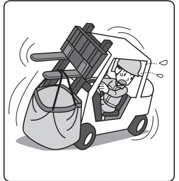
**3** Watch out for overloading and load collapse!
