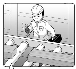
Prior to starting an inspection, make sure that the machine has come to a complete stop.
