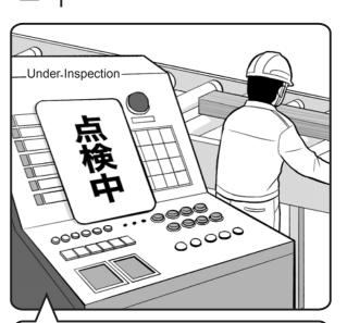
Put a sign up when stopping a machine to handle a problem.
