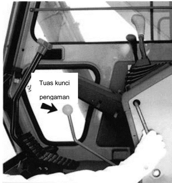
Gambar 3-5 Contoh safety lock lever (tuas kunci pengaman atau safety lock lever)
