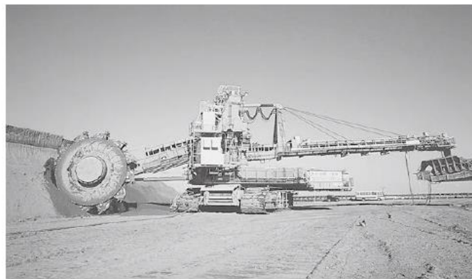
Litrato 1-11 Bucket Excavator
