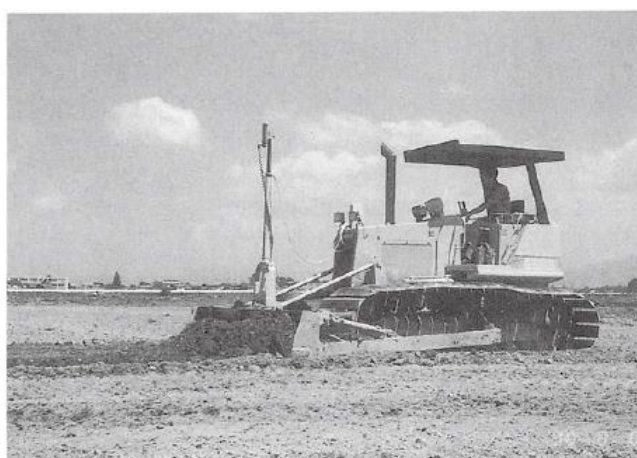
Litrato 6-4 Halimbawa ng Blade Control Device
