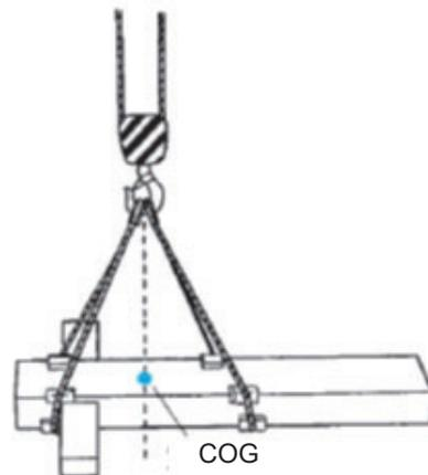
**Fig. 5-20** Slinging with correct COG location
