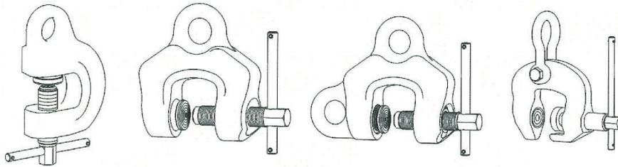
**Fig. 3-14** Screw-type clamps
