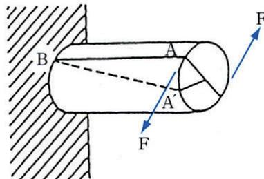
**Fig. 2-21** Twisting Load
