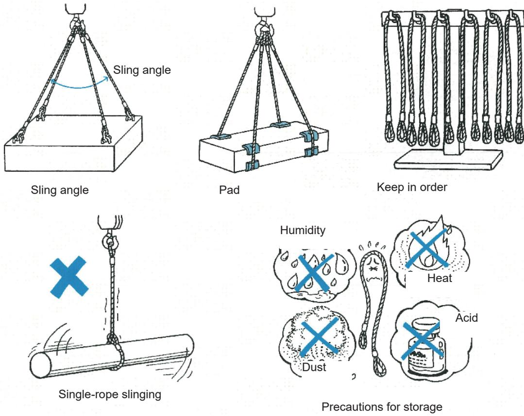
**Fig. 3-9** Precautions when Using Sling Wire Rope
