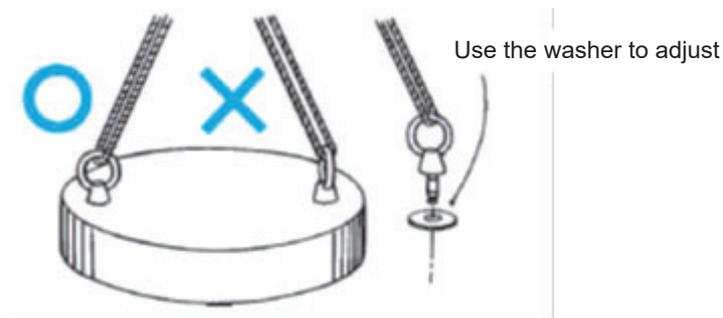
Fig. 3-24 Example of Using Eyebolts
