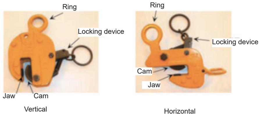
**Fig. 3-13** Cam-type clamps
