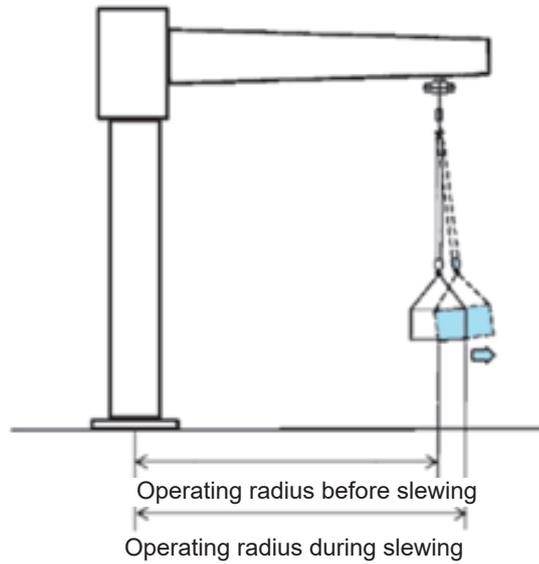
**Fig. 2-12** Outward Movement of Lifted Load and Changes in Operating Radius due to Centrifugal Force
