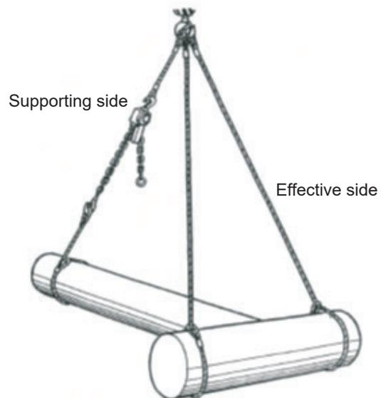
**Fig. 5-23** Slinging adjusted with another hoisting accessory: Effective side: Fastening by eyes
