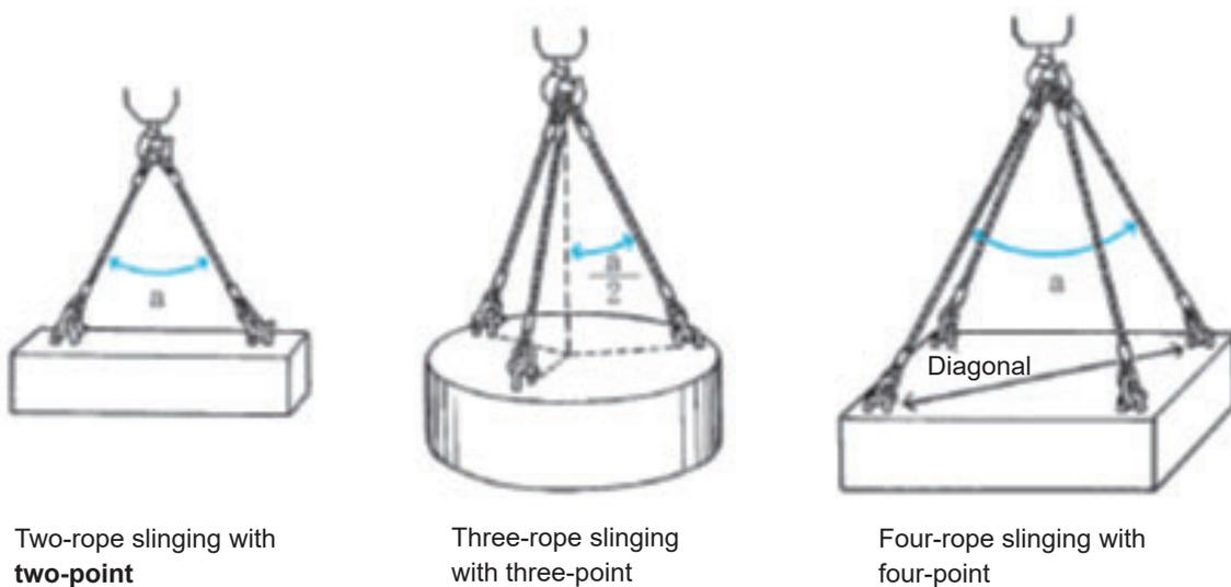
**Fig. 2-24** Number of Ropes and Sling Angle (a = Sling angle)
