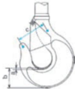
Fig. 3-38 Opening and wear of hooks
