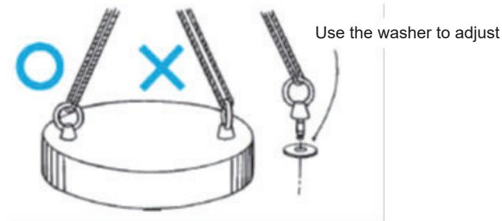
Fig. 3-24 Example of Using Eyebolts
