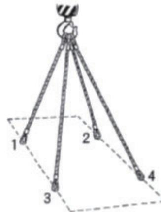
**Fig. 5-15** Lengthwise direction is perpendicular to the direction of the hook (1-3-2-4 or 3-1-4-2 from hook end)
