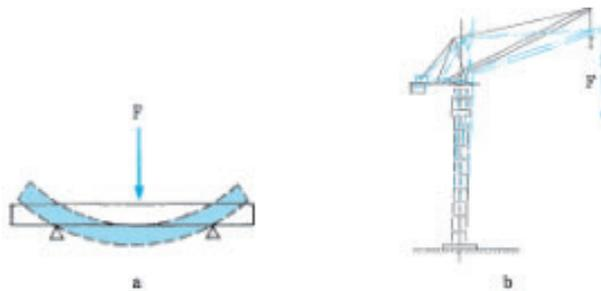
**Fig. 2-20** Bending Load
