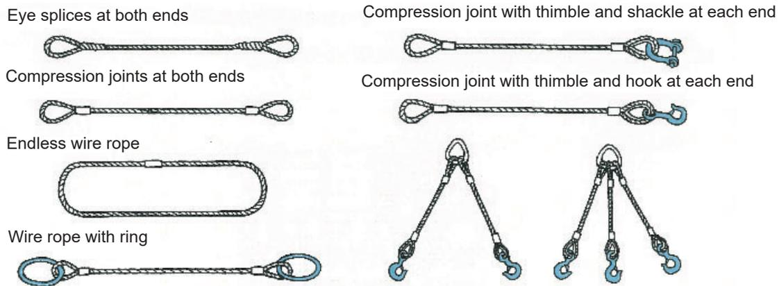
**Fig. 3-7** Sling Wire Rope
