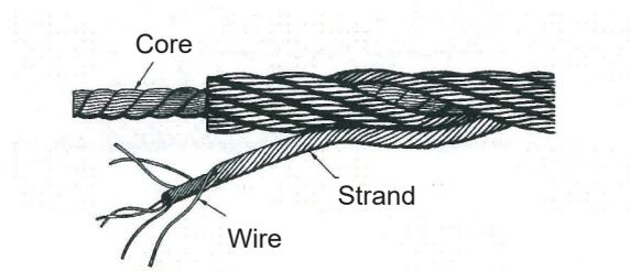
Fig. 3-1 Construction of Wire Rope
