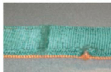
Fig. 3-33 Damage on the end loop
