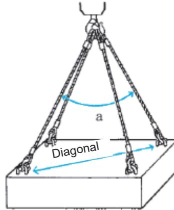
Fig. 3-6 Sling Angle for Four-rope Slings with Four-point
