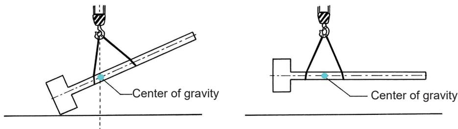
Fig. 5-3 How to Determine the Location of the COG during the Work
