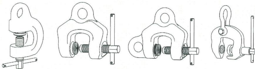
**Fig. 3-14** Screw-type clamps
