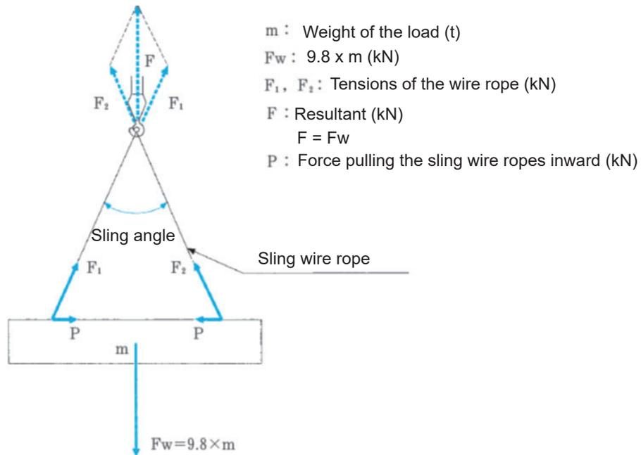
Fig. 2-25 Tension of Sling Wire Ropes
