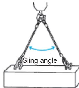
**Fig. 3-4** Sling Angle for Two-rope slinging with Two-point
