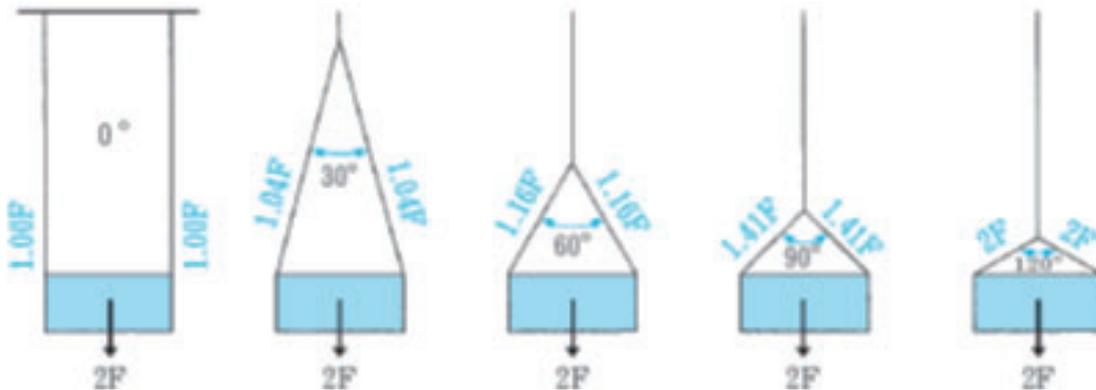
Fig. 2-26 Relationship between Sling Angle and Tension
