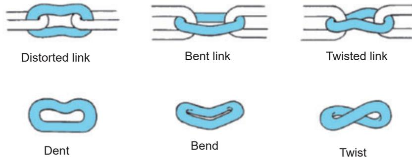
**Fig. 3-29** Deformation of Chain
