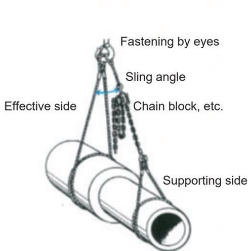
**Fig. 5-22** Slinging adjusted with another hoisting accessory: Effective side: One-round-turn slinging
