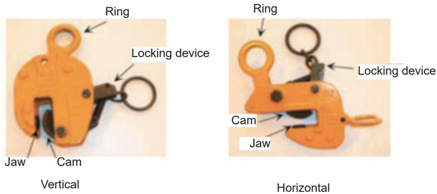
**Fig. 3-13** Cam-type clamps
