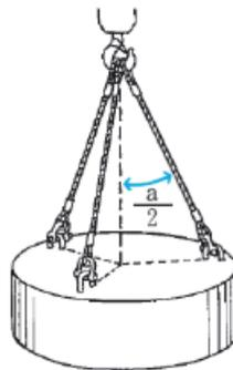
**Fig. 3-5** Sling Angle for Three-rope Slinging with Three-point
