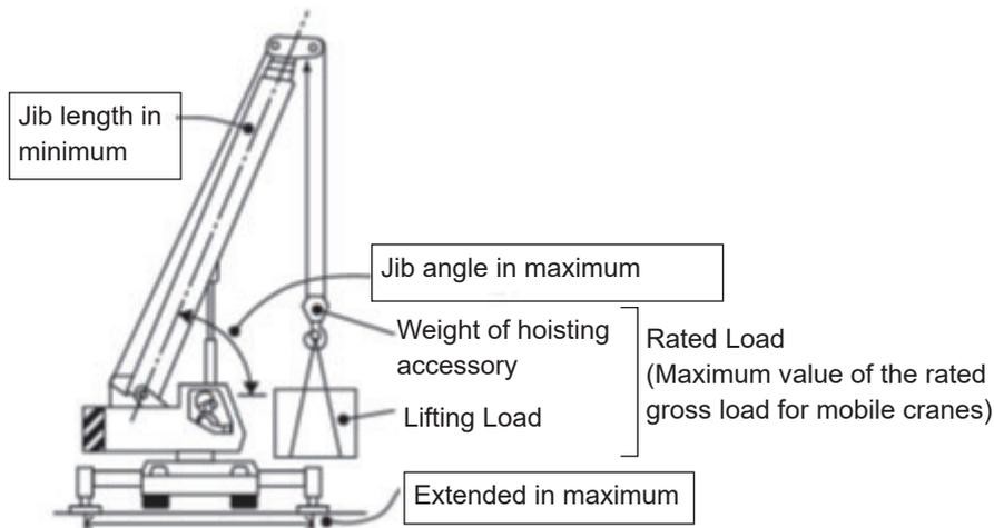
**Fig. 1-5** Relation Between Lifting Load, Rated Gross Load, and Rated Load
