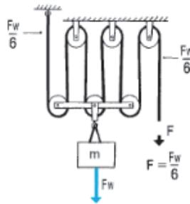
**Fig. 2-15** Combination Pulley (Three Movable Pulleys)
