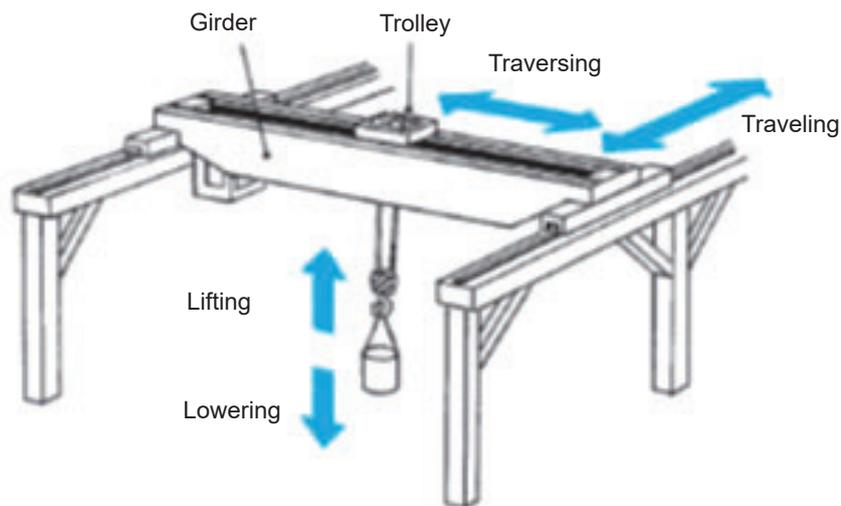
**Fig. 1-1** Lifting, Lowering, Traversing, Traveling
