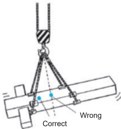
**Fig. 5-19** Slinging with COG locating error
