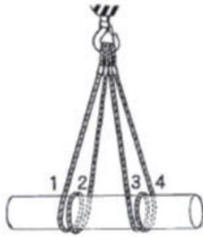
**Fig. 5-16** Lengthwise direction is parallel to the direction of the hook (1-2-3-4 from hook end)
