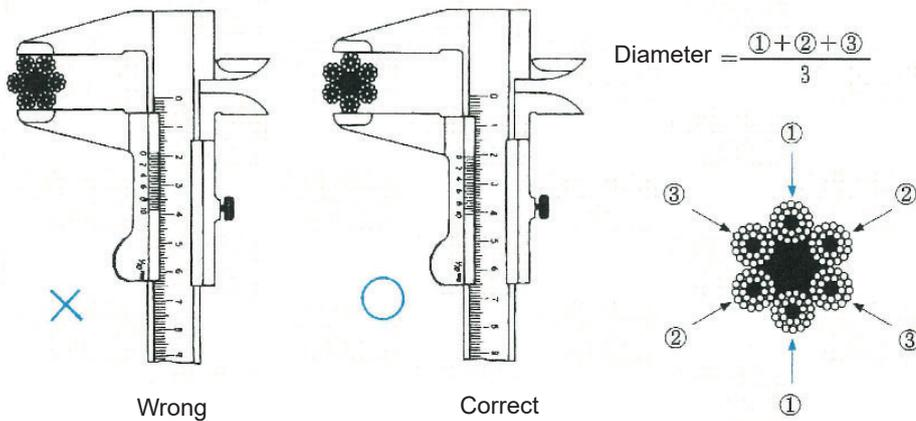
Fig. 3-3 Measuring Method for Diameter of Wire Rope
