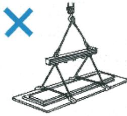
Do not use hackers when lifting stacked items with different dimensions.
