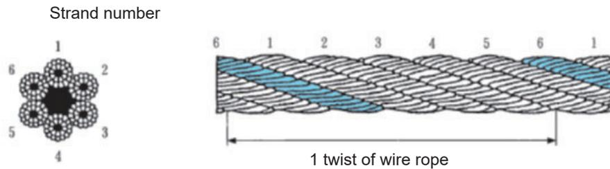
**Fig. 3-27** 1 twist of wire rope
