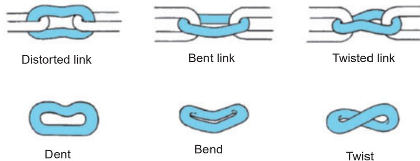
**Fig. 3-29** Deformation of Chain
