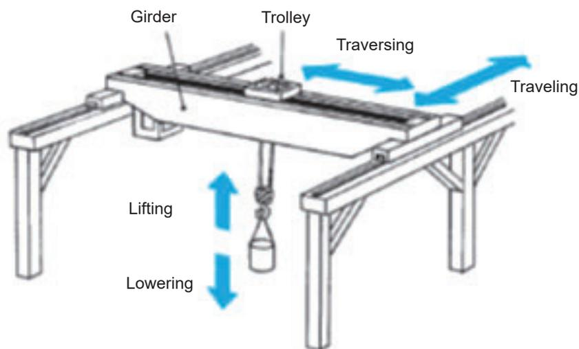
**Fig. 1-1** Lifting, Lowering, Traversing, Traveling
