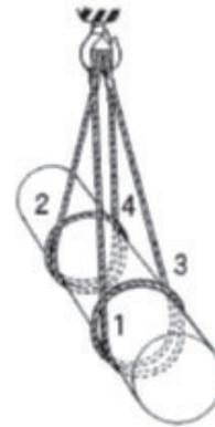
**Fig. 5-17** Lengthwise direction is perpendicular to the direction of the hook (1-2-3-4 or 2-1-4-3 from hook end)
