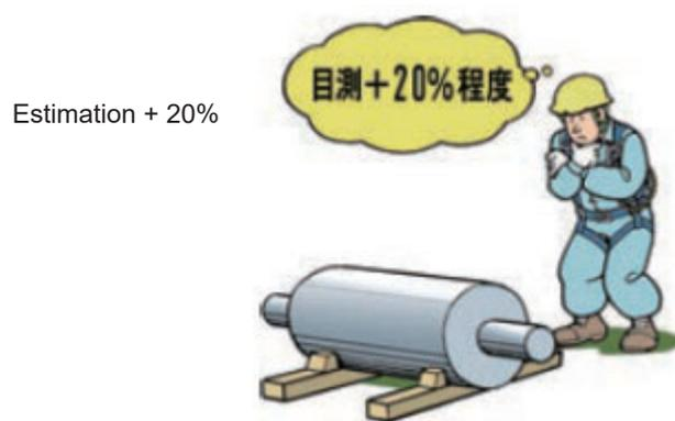
**Fig. 5-2** Estimate the Weight of the Load
