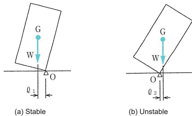
Fig. 2-8 Stability of Material Body
