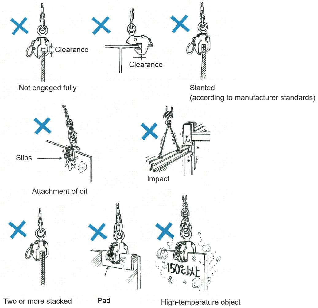
**Fig. 3-15** Unacceptable Method to Sling with Clamps
