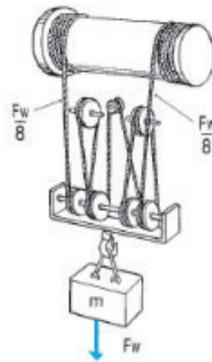
**Fig. 2-16** Combination Pulley (Four Movable Pulleys for Crane)
