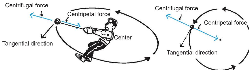
Fig. 2-11 Centripetal and Centrifugal Forces
