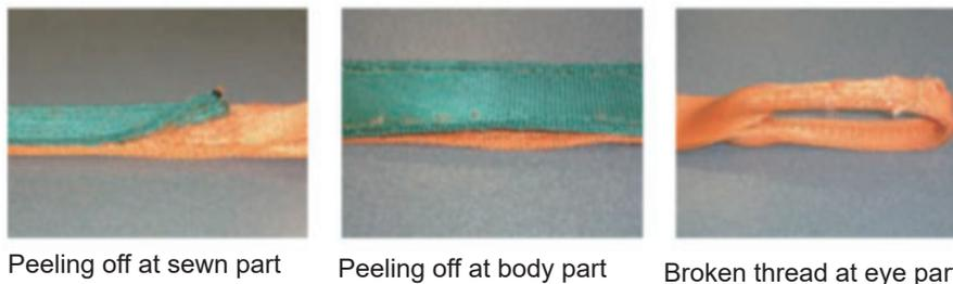
Fig. 3-31 Peeling off at belt
