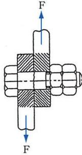
**Fig. 2-19** Shearing Load
