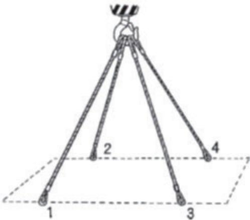
**Fig. 5-14** Lengthwise direction is parallel to the direction of the hook (1-2-3-4 or 2-1-4-3 from hook end)
