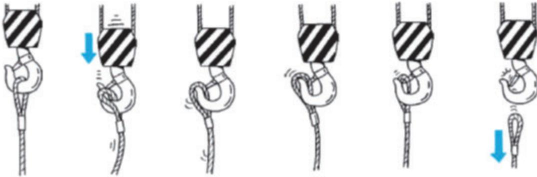
**Fig. 5-13** How an eye comes out from a hook
