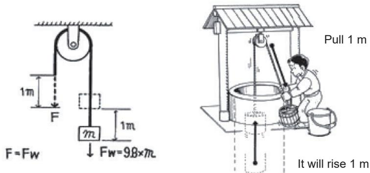
Fig. 2-13 Stationary Pulley
