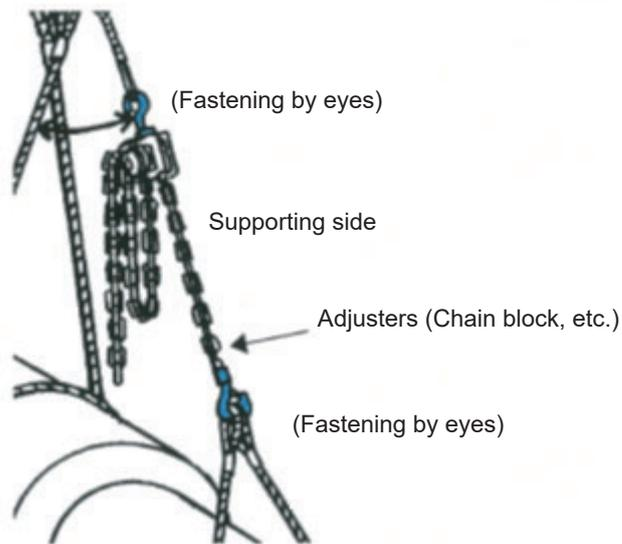
**Fig. 5-24** How to Attach the Adjusters
