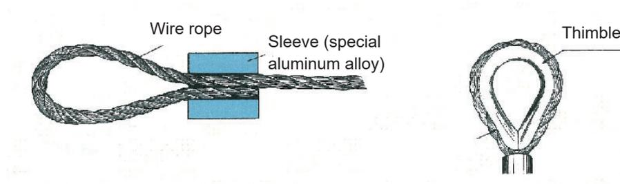
**Fig. 3-8** Compression Jointing Method
