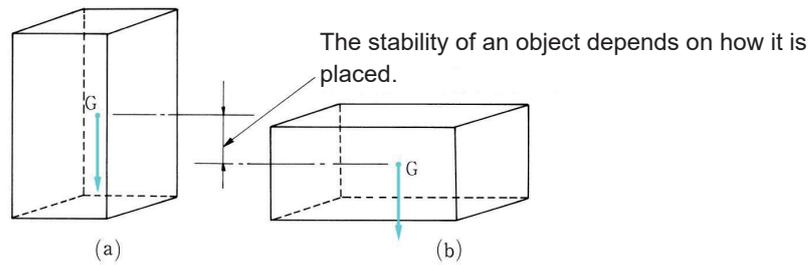
**Fig. 2-9** Stability of Material Body when Placed in Different Way
