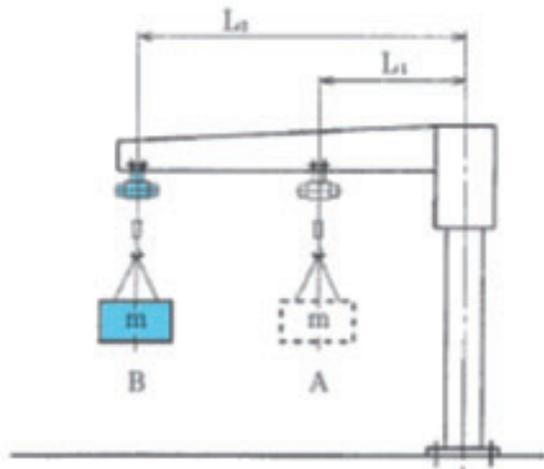
**Fig. 2-5** Moment Working on Jib Crane
