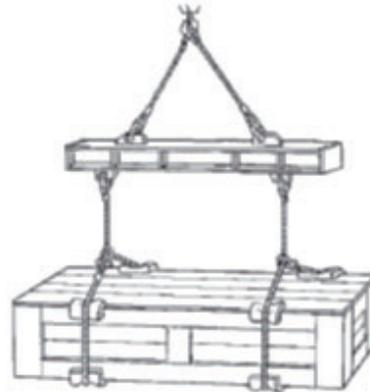
**Fig. 5-10** Slinging with lifting beam
