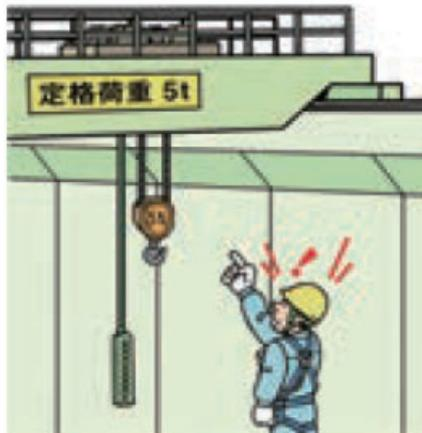
**Fig. 5-1** Display example of rated load on overhead traveling crane
