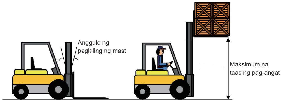
Fig. 1-3 Mast tilt angle at maximum na taas ng lift
