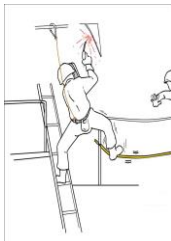
Do not step on the railings
