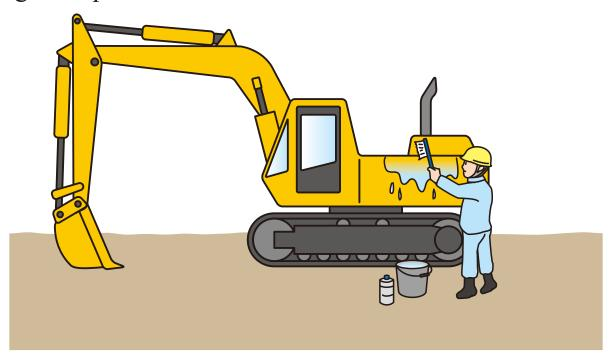
2. After the work is completed, park the machine in a designated place, lower the work equipment to the ground, and then stop the engine. When the engine is stopped, all operation levers should be "neutral" and locked. After unplugging the machine, store it in a designated place.
