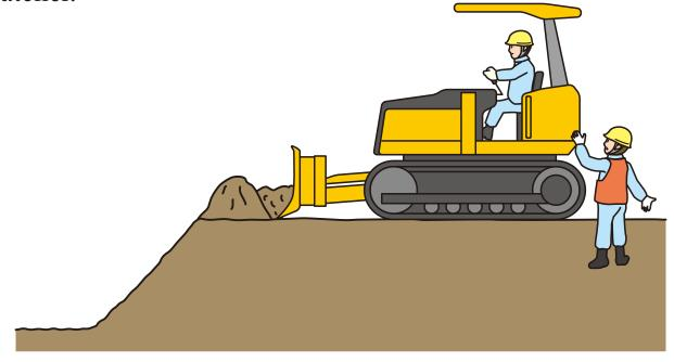
2. In the soft ground, do not use control levers too much (do not turn). Also, use a swamp bulldozer and avoid running in the same place as possible.
