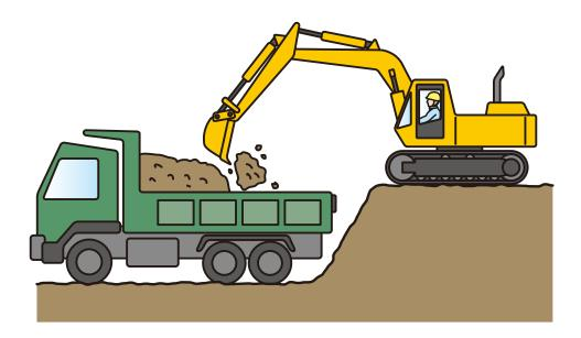
2. When loading on a dump truck, the arm must turn from the backside of the driver's cabin, not above the driver's cabin.
