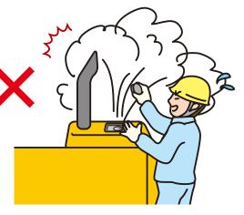
When the radiator is hot, be aware that hot water may blow out if the cap is removed.
