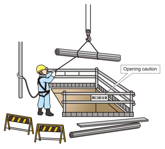
When removing handrails/middle bars of the openings, a personal fall arrest system (fall prevention harness) is required and never hook it to the handrail. In addition, do not go up and down by using a handrail or a middle rail as a step.
