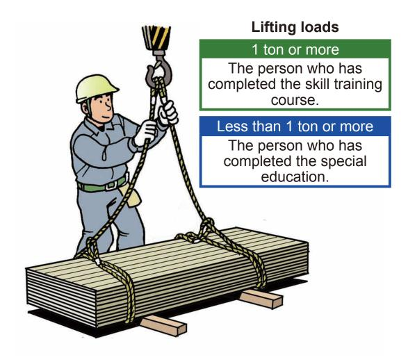
"Lifting loads" is not the weight of the suspended loads, but the lifting loads of a crane or a mobile crane used.
