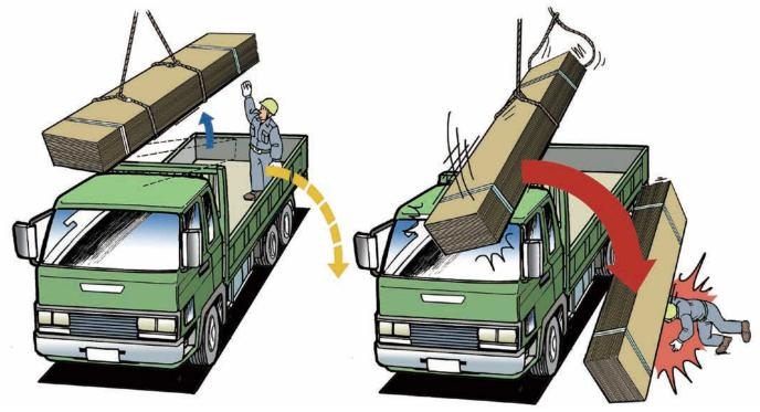
When hanging a suspended load with two wire ropes and tried to lift it.
