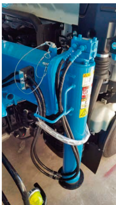
Outrigger lock pin and an example of the pop-out preventive chain
