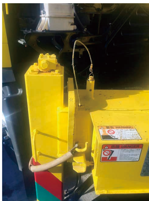
Outrigger lock pin and an example of the pop-out preventive chain
