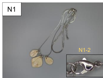
Niの溶出量が 0.5 \mu\text{g}/\text{cm}^2/\text{week} を超えた試料例
