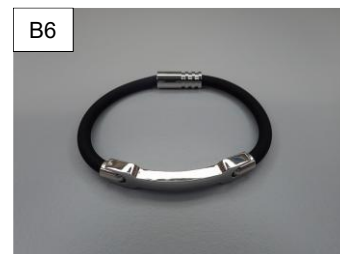
Niの溶出量が 0.5 \mu\text{g}/\text{cm}^2/\text{week} を超えた試料例
