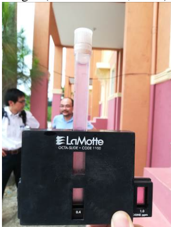
Sampling point at San Jose Del Monte Water District. Test for residual Cl with colorimetric method. COWD uses the same method. (November 27, 2017)
