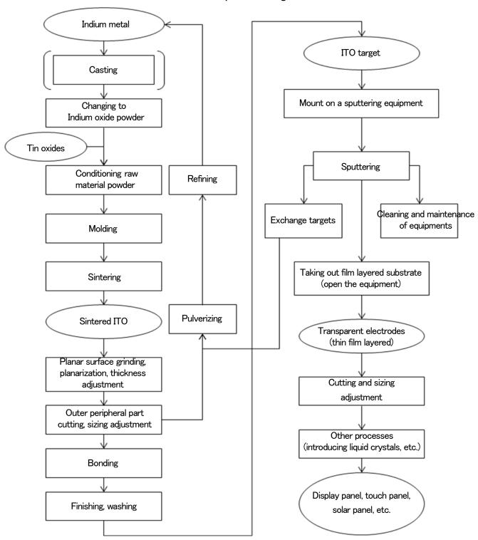
Note: Sputtering is a method wherein high voltage is applied to the gap applied between substrate and target while introducing inert gas into a vacuum, and bombarding the target with a beam of ionized inert gas to eject atoms from the target surface to form a thin layer of the same substance on the substrate.
