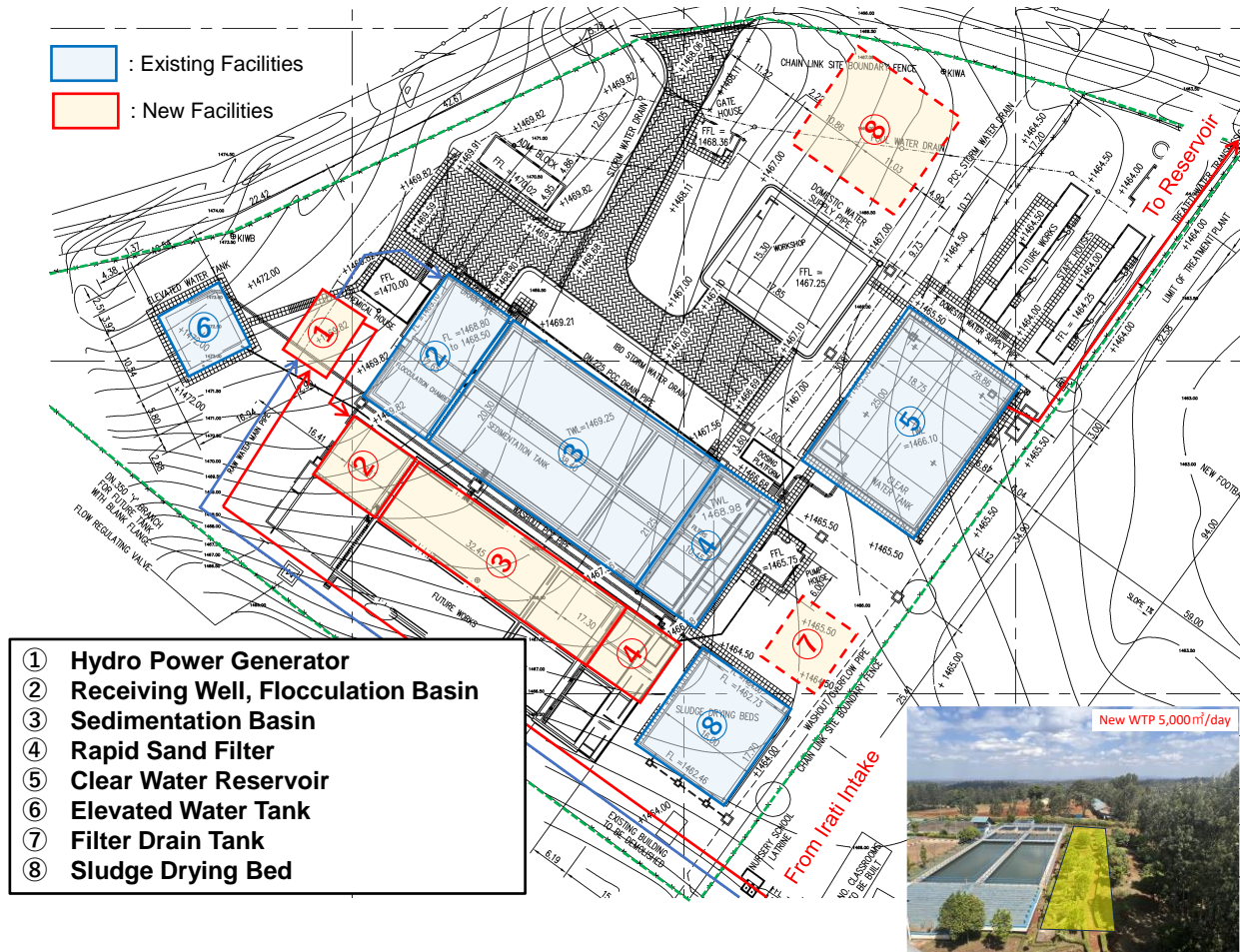
Figure 3-5 Image of the Expansion of the Kiawambeu WTP
