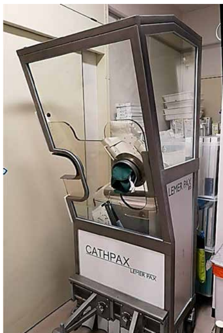
Fig. 5 Radiation protection cabin
