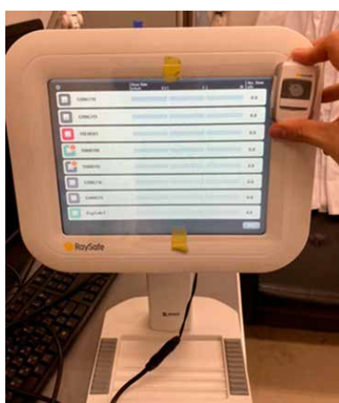
Figure 2. A schematic of the i3 system (left: base station with 10.4-inch display; right: i3 dosimeter sensor). The system comprises a wireless i3 sensor (solid-state semiconductor detector) that transmits the scattered-radiation dose to the base station. The i3 sensor is small (40 × 58 mm, 34 g) and thus easy to carry during interventions.
