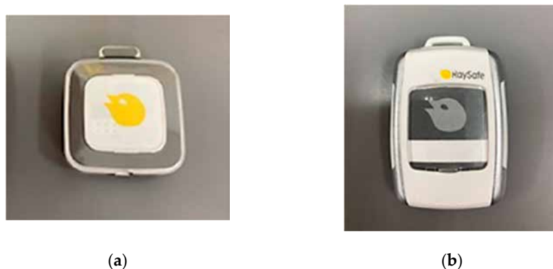
Figure 1. (a) The RaySafe i2 sensor (44 × 45 mm); (b) The RaySafe i3 sensor (40 × 58 mm). Recently, the i3 sensor has replaced the former i2 sensor.
