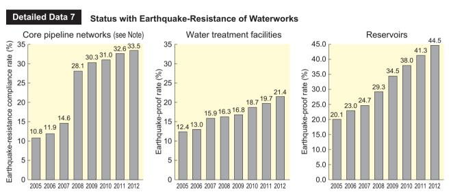
(Note) The figures indicate the percentage of pipes that were earthquake-resistant (earthquake-proof rate) up to FY2006 and the percentage of pipes that meet earthquake-resistance standards (earthquake-resistant pipes + non-earthquake-resistant pipes but which are situated in better ground and are therefore considered to be earthquake-resistant) (earthquake-resistance compliance rate) from FY2007 on.
