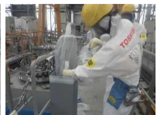
The new survey meter can measure \beta -rays with a single measurement, using a single unit.
