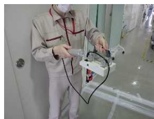
The new survey meter can measure \beta -rays with a single measurement, using a single unit.
