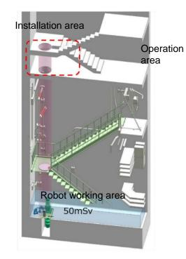
The robot was installed from the opening on the ground floor.
