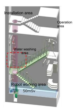
When taking the robot from the basement floor, it was cleaned with high-pressure water.
