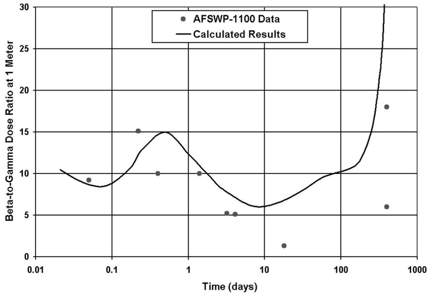
Fig. 6. Comparison of calculated and measured beta-to-gamma dose ratios.
