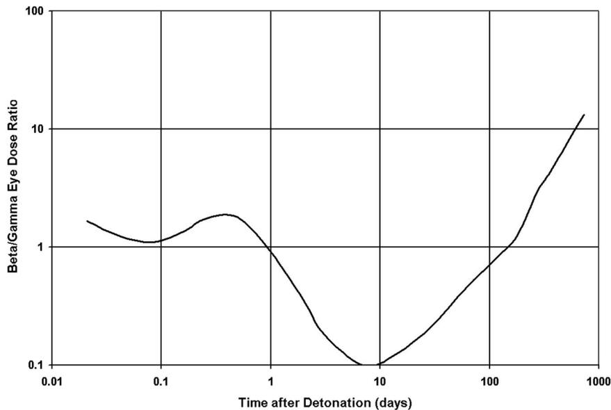
Fig. 7. Time dependence of beta-to-gamma eye dose ratios for Pacific test site exposures.
