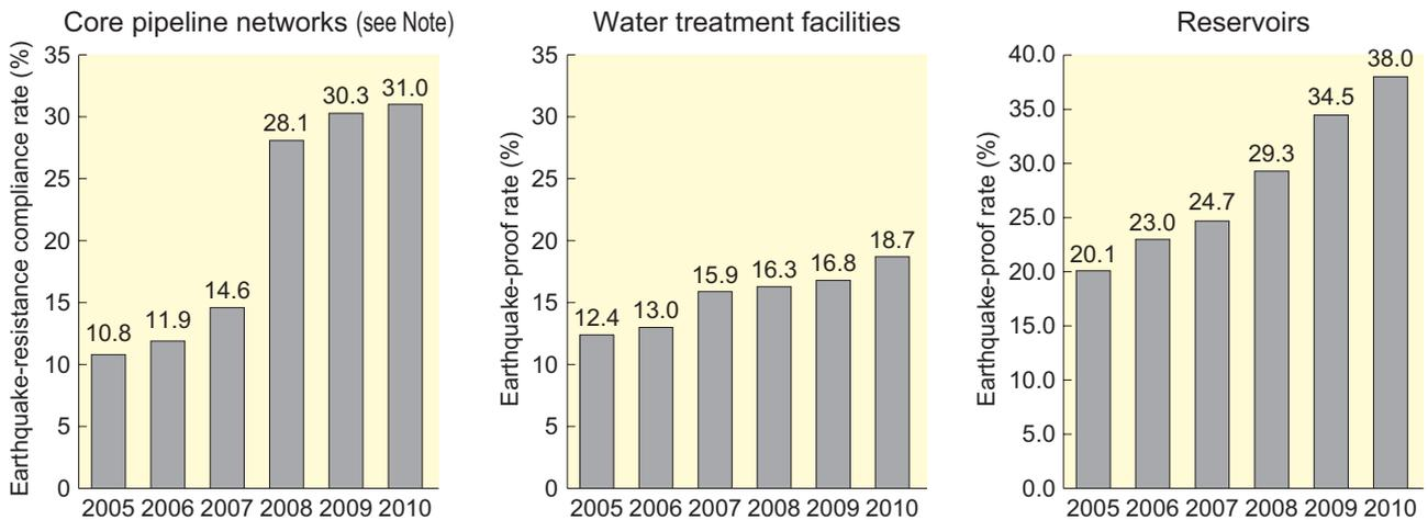
(Note) The figures indicate the percentage of pipes that were earthquake-resistant (earthquake-proof rate) up to FY2006 and the percentage of pipes that meet earthquake-resistance standards (earthquake-resistant pipes + non-earthquake-resistant pipes but which are situated in better ground and are therefore considered to be earthquake-resistant) (earthquake-resistance compliance rate) from FY2007 on
