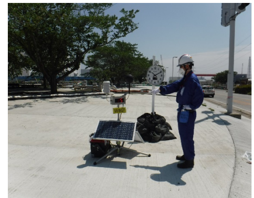
Deployment of WBGT indicator and clock
