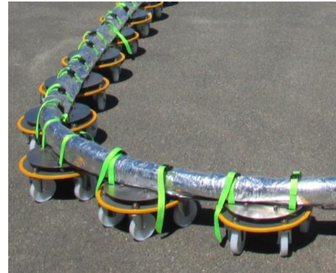
A suction hose and the wheeled platform
