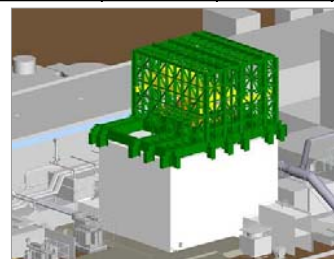
Frame for Unit 1 pool
