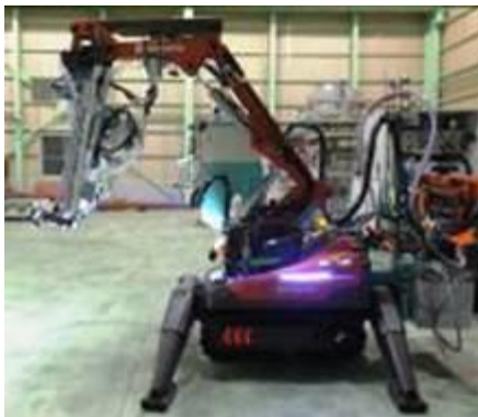
Middle-upper decontamination equipment (remodeled small heavy equipment)
