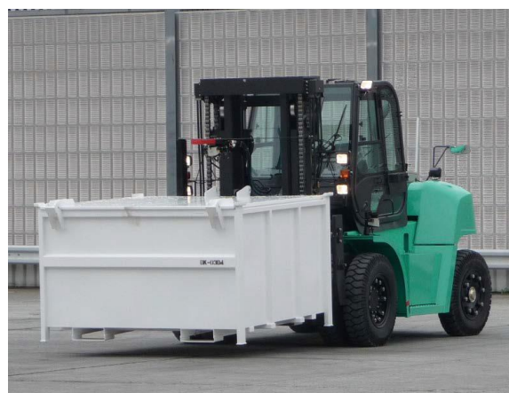
Unmanned forklift for transporting high dose rubble
