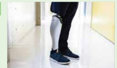
A powered prosthesis that assists persons with a lower limb amputation to move their legs, developed in the Project for Promoting the Development of Equipment to Support Independence for Persons with Disabilities
